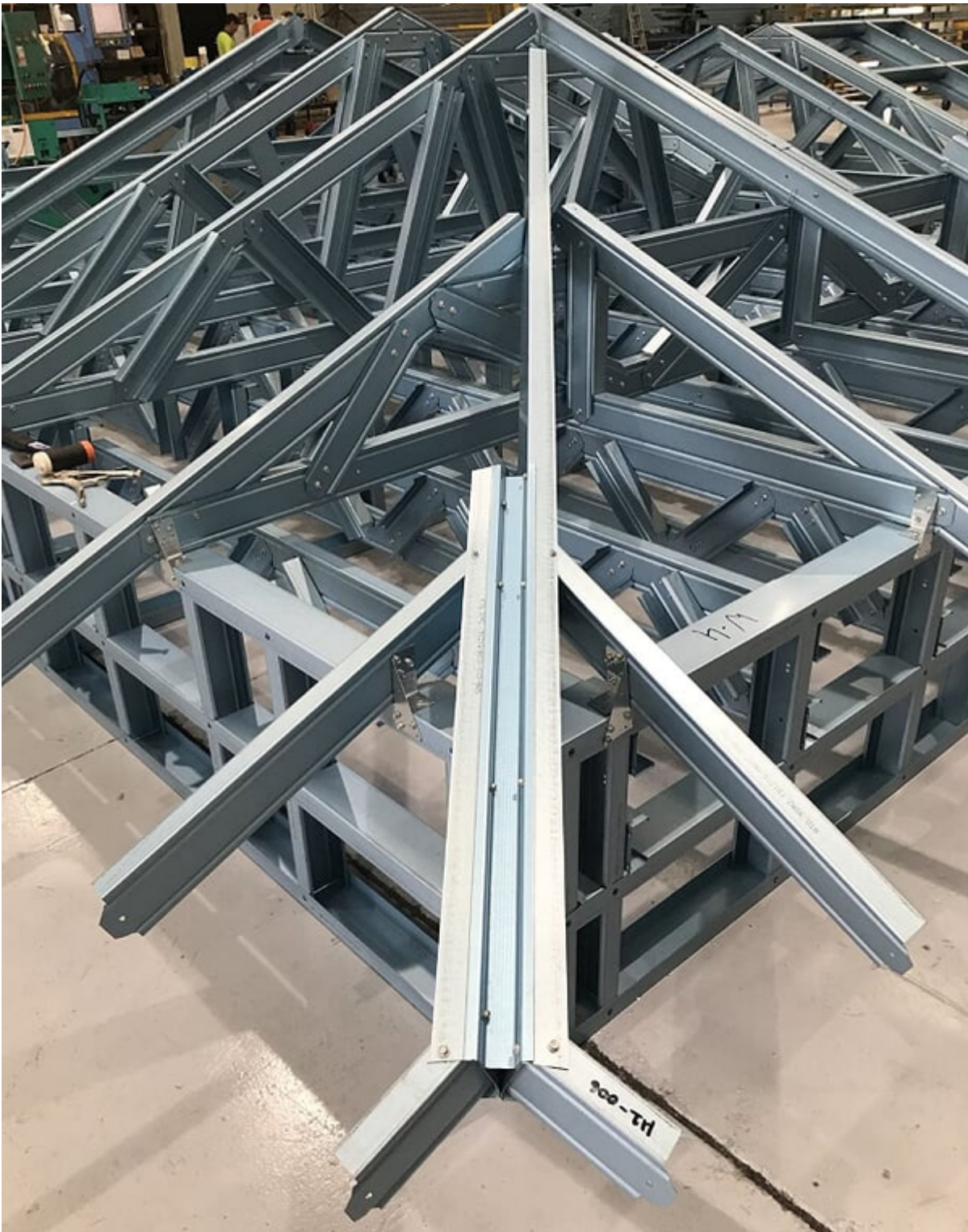
Figure 7.34: Installed veed hip rafter with creeper rafters bent out
