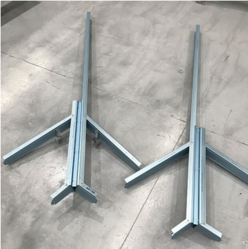
Figure 7.32: Left and right veed hip sections
