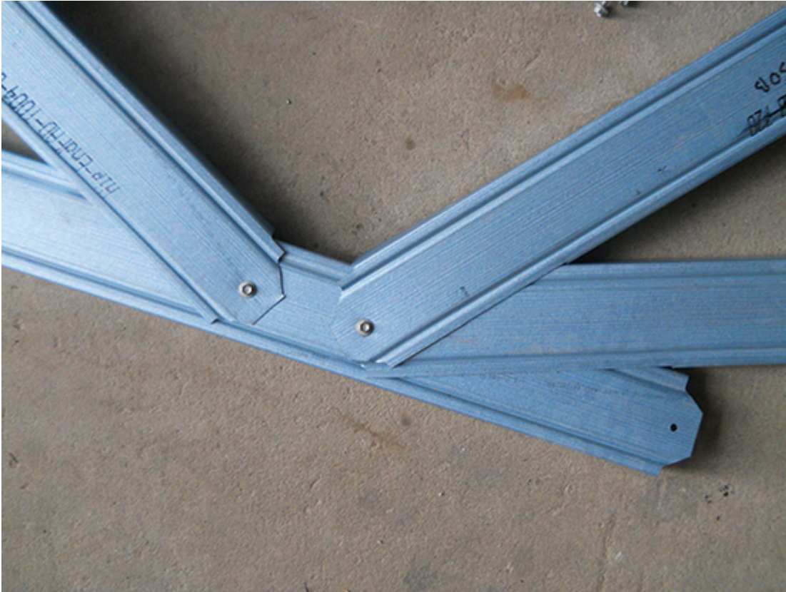
Finished knee web connection (unreinforced)
