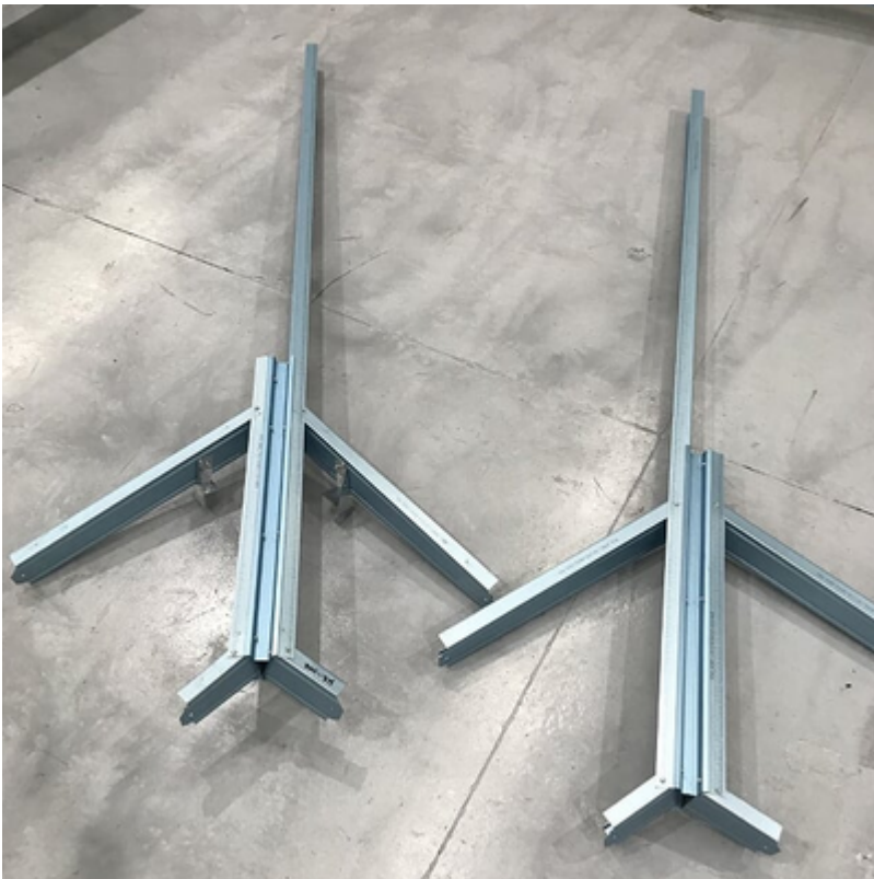
Figure 7.32: Left and right veed hip sections
