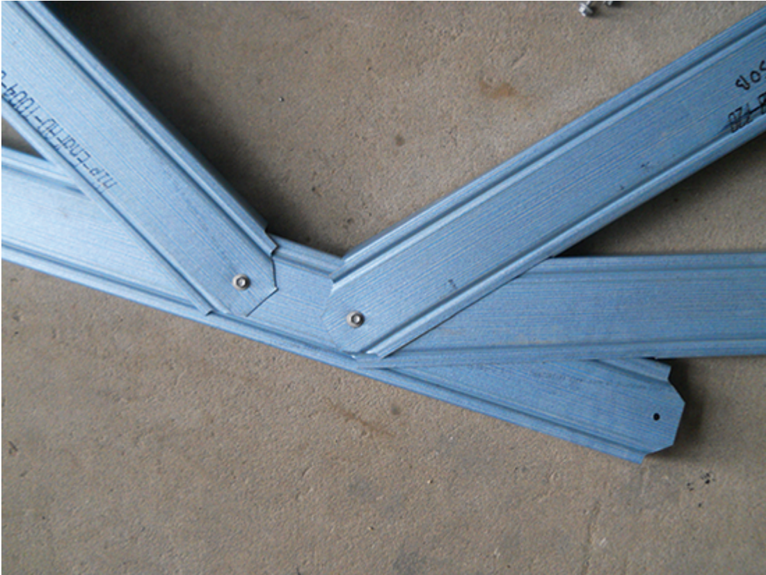
Finished knee web connection (unreinforced)
